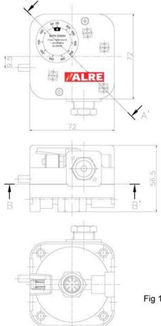
Fig 1. Gas pressure switch(V)
